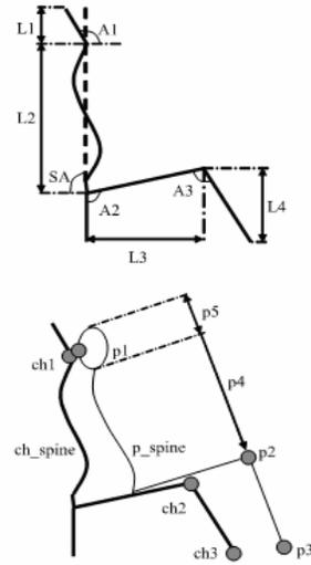
**Figure 1. (a) chair design parameters (b) objective function parameters**
