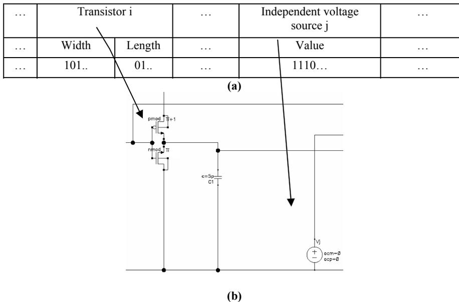
**Figure 2. a) Chromosome and b) the parameters of the circuit elements, created from it**
