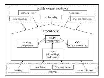
Figure 1: Scheme of Greenhouse Climate Model
