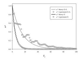
Figure 5: The error  $\alpha$  for G and G+L as a function of the allowable time  $T_a$  shows good agreement between theory and experiment and also demonstrates the correctness of the optimality condition. In this case, G should be used alone, because it consistently gives lower error for the same allowable time.
