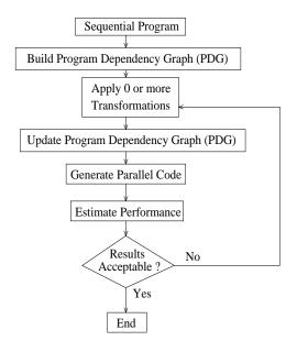
Figure 1: Typical Automatic Parallelization Process
