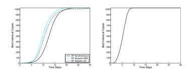
Left part: Growth curves for synchronous, and two asynchronous update policies. Initial best individual uniformly distributed among the nodes.
