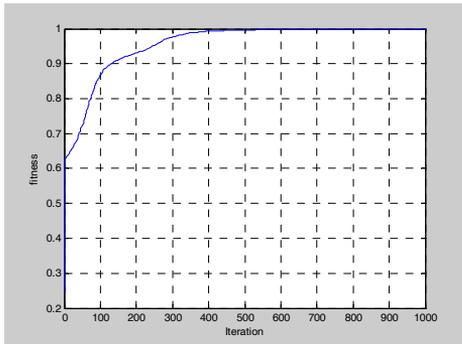
**Figure 8. Learning curve, the relation between fitness and iteration of the forth order equalizer**
