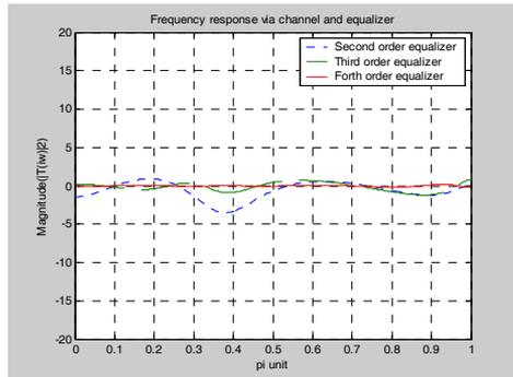
**Figure 10. Frequency response via channel and three equalizers**
