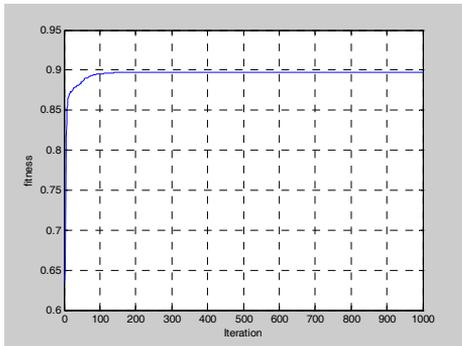
**Figure 6. Learning curve, the relation between fitness and iteration of the second order equalizer**
