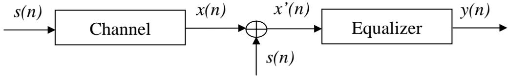
**Figure 5. Simplified Model of a Communication System with AWGN noise**
