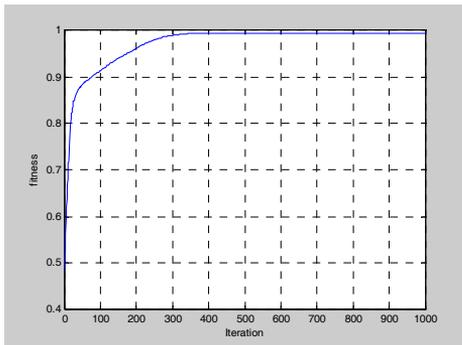
**Figure 7. Learning curve, the relation between fitness and iteration of the third order equalizer**
