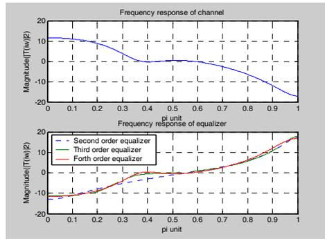
**Figure 9. Frequency response of the channel and equalizers**
