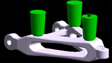
¬ Feeder Volume before: about 0.93 l after: about 0.46 l 126 calculated designs Calculation time 3<sup>1</sup>/<sub>2</sub>h
