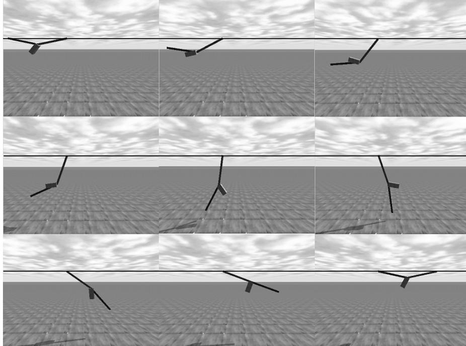
**Fig. 2.** This is a series of screenshots from the Open Dynamics Engine™ simulation. The steps are evenly spaced starting at  $t = 0$  and ending at  $t = 1.335$ . This particular brachiator can travel 167 meters over the course of 60 swings, with an efficiency of 0.26 meters/joule.
