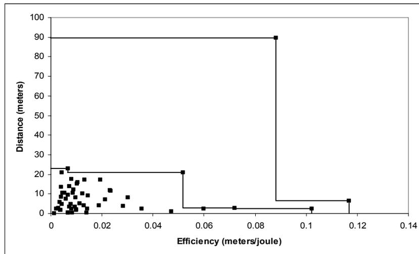
**Fig. 3.** The brachiators selected for reproduction lay on the first and second Pareto optimization curves. Two curves were used as to not so severely limit the gene pool. This particular data is from the first generation of randomly generated brachiators. There are roughly 50 brachiators represented here – the rest failed to even swing once for a positive distance.
