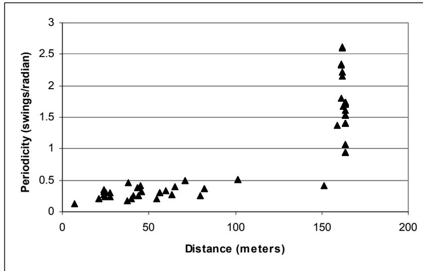
**Fig. 4.** A scatter plot showing periodicity vs. distance brachiated for a population of 100 brachiators after 53 generations. While not all of the long-distance brachiators exhibit high levels of periodicity, they are the only group that does.
