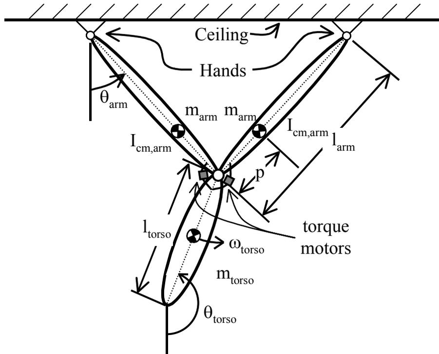
**Fig. 1.** The three rigid bodies that make up the brachiators consist of two arms and a trunk, which all connect at a common shoulder. Torque is created between the arms and the body by torque motors, which are controlled by the torque function stored in the genome. Note that the centers of mass for the two arms do not lie in the centers of the arms. Also, the ceiling contains an infinite number of handholds, not just the pin joints shown.
