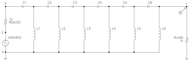
Figure 1 Best-of-run circuit when inputs call for a highpass filter.
