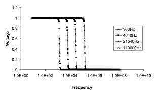
Figure 7 Frequency domain behavior of best-of-run circuit for four out-of-sample values of frequency when inputs call for a lowpass filter.
