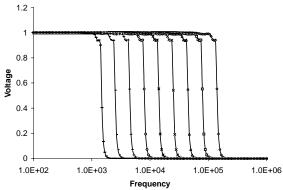
Figure 4 Frequency domain behavior of best-of-run circuit when inputs call for a lowpass filter.
