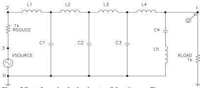
Figure 2 Best-of-run circuit when inputs call for a lowpass filter.
