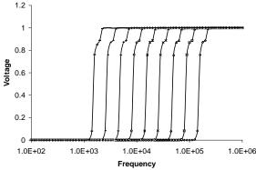
Figure 3 Frequency domain behavior of best-of-run circuit when inputs call for a highpass filter.
