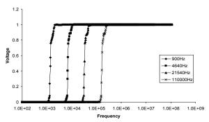
Figure 6 Frequency domain behavior of best-of-run circuit for four out-of-sample values of frequency when inputs call for a highpass filter.
