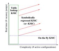
FIG. 1: Schematic illustration of simulation capabilities and bottlenecks of on-the-fly KMC, table look-up KMC, and symbolically-regressed KMC (sr-KMC).
