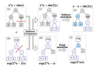
FIG. 2: Illustration of tree representation, subtree crossover, subtree mutation, and point mutation used in GP.
