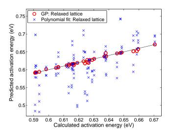
FIG. 4: Activation energies (in eV) predicted by regression. GP (circles) and a quadratic polynomial (crosses) are compared to the calculated (Morse) barriers for  $1^{st}$  n.n. jumps on (100)-surface of Cu<sub>0.5</sub>Co<sub>0.5</sub> for relaxed lattices. As a simple test, only first n.n. environments are considered in the active configuration. The line is a guide for the eye.
