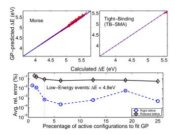
FIG. 5: (Upper) Calculated vs. GP-predicted barriers (in eV) for 2<sup>nd</sup> n.n. jumps on relaxed (100)-surface of Cu<sub>0.5</sub>Co<sub>0.5</sub> active configurations up to 2<sup>nd</sup> n.n. for Morse and TB-SMA. (Lower) GP predicts the barriers with 0.1% (1%) error for most- (less-) significant events with  $\Delta E < 4.8$  eV ( $\Delta E > 4.8$  eV) from only 3% of active configurations.
