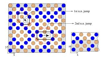
FIG. 3: Sketch of simulation cell for vacancy-assisted migration on (100)-surface of an fcc binary alloy. Atoms in all but the bottom layers and the boundary can fully relax. The solid (dashed) lines around the migrating atom and vacancy represent  $1^{st}$  (2<sup>nd</sup>) n.n environmental atoms.
