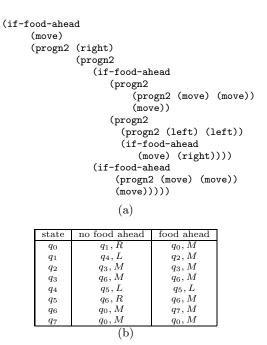
Figure 5: An example of genetic programming result (a) evolved S-expression  $(n_t = 12, n_f = 4)$  (b) converted FSM
